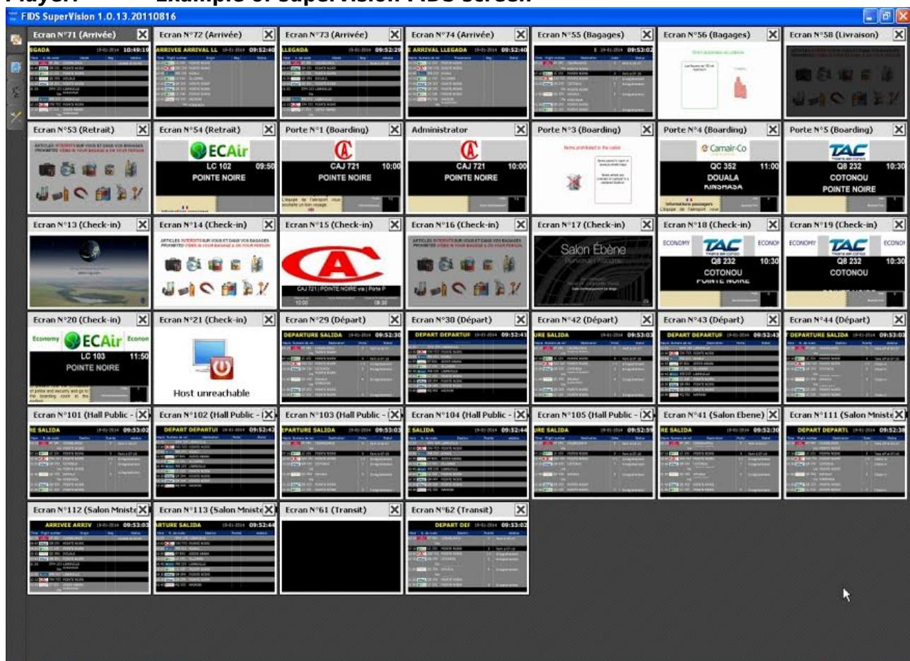
**SuperVision allows administration of several platforms. It can be used in two modes for Edge-airport solutions: - supervision of the Cupp-T system (IATA CUPPS platform); - . supervision for FiDS , flight information display system.**
