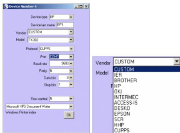
Just select a vendor and model from the list of CUPPS certified hardware to add or replace a device (Boarding pass or boarding tag printer, passport reader, magnetic card reader, etc.).
